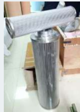
Jacking Oil Filter
